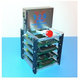
Fig. 9. Prototype CubeSat Card Cage design.
