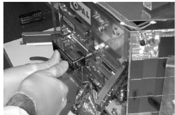
Figure 2.6 Loading a Picosat into OPAL
